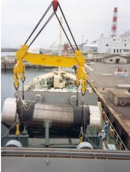
Fig. 4.3.19 Loading a container with spent fuel on a ship, Japan (photo John Mairs/IAEA)
