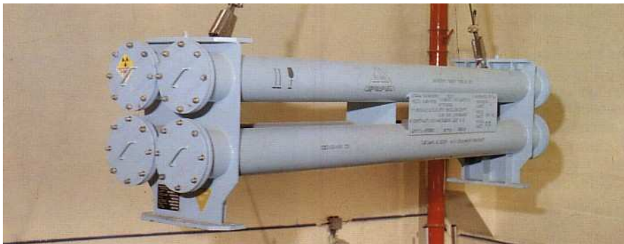
Fig. 4.3.10 Fresh fuel transport container to pressurized water reactors of Russian construction, type WWER-440.[Imatran Voima Oy: Loviisa Power Plant]
