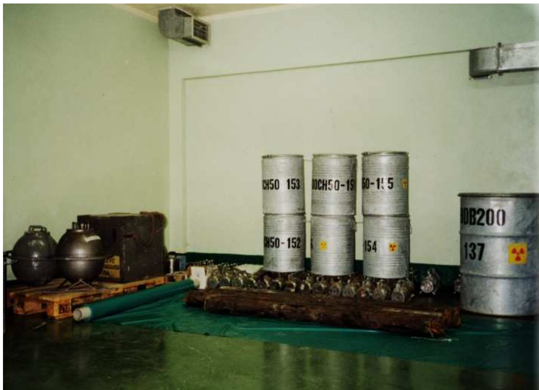
Fig. 4.3.27 Low level radioactive waste prepared for transport to the storage [ZUOP Świerk].
