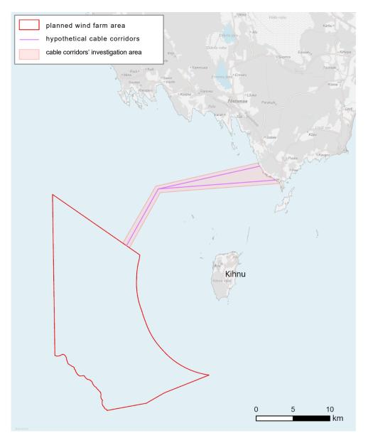
Figure 2-3. The hypothetical cable corridor locations in the sea for connecting the planned Saare-Liivi wind farm
