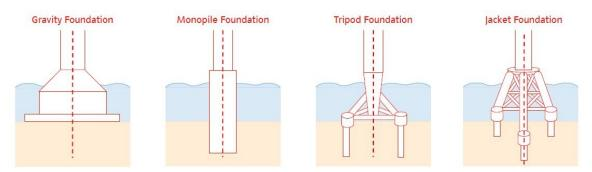
Figure 2-2. Types of electricity turbine foundations used in offshore wind farms<sup>117</sup>
